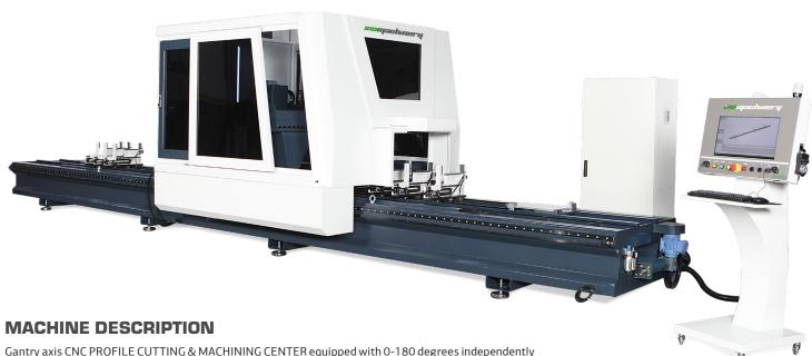
programmable high speed spindle, 45-90-135 degrees automatically tilting sawblade with 600 mm diameter, automatic tool changer magazine, 12 profile clamping devices, pneumatic referance pins and 3D programming software.
